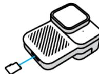
You can eject the card by pressing it into the slot with your fingernail.
